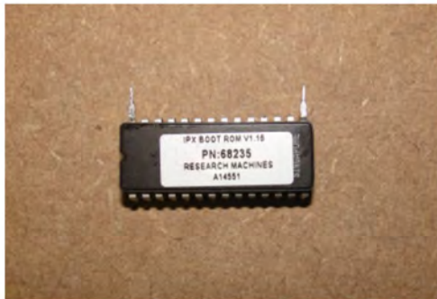
Figure 2 - PN:68235 IPX BOOT ROM chip with pins 1 st and 14 th bent outward
